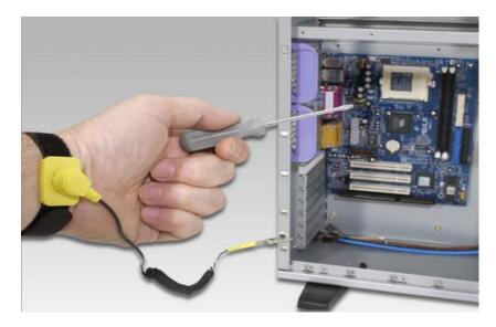
Figure 1: Static Protection Wrist Strap
